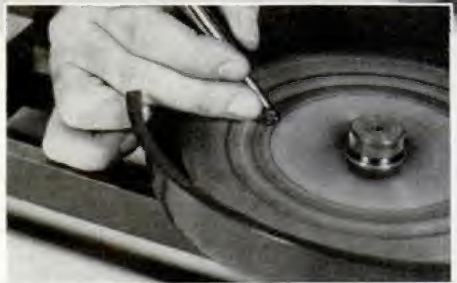
LAP PLATE can be of copper, tin or plastic, depending on faceting step. Pie tin acts as splash guard
